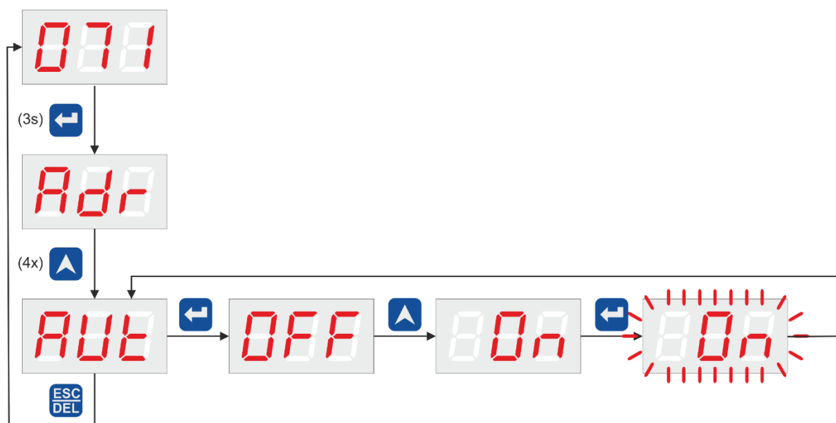
Fig. 16 The automatic test of the optical system configuration.
